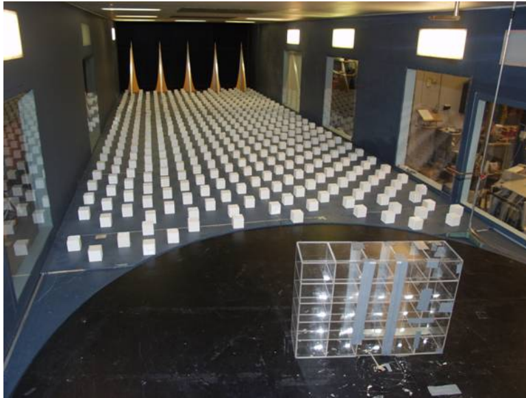
Figure 6.2 The building model placed in the wind tunnel in Gävle, Sweden.
